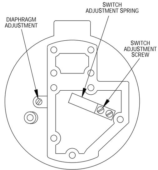
The **Series P/G Ultra Mag™ Level Switch** provides level indication by detecting pressure applied by the bulk material to the sensing diaphragm. The switch is tripped magnetically, as the result of 2 magnets with like poles repelling one another. The fields of the magnets perform through the nonferrous wall of the switch housing. Pins, links and "O" rings, which often cause failure due to moisture, dirt, and corrosion, are eliminated. The switch enclosure is completely sealed.
