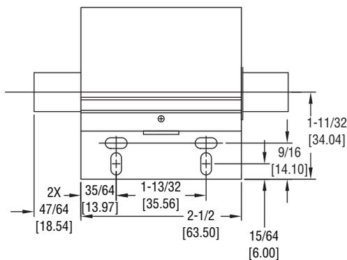
Figure 2: Mounting Hole Dimensions
