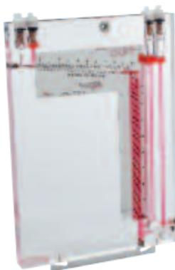
1. Mount gage securely on a vertical surface avoiding excessive heat. (Temperatures over 150°F (65.6°C) will damage gage). Level gage approximately by swinging gage about top center mounting screw and locate bottom bracket screws in center of slots.
